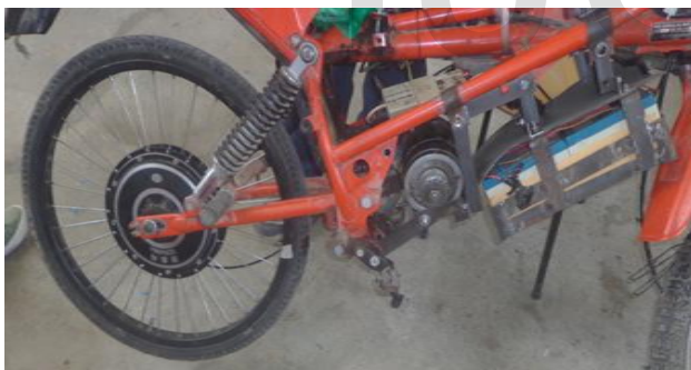
Figure 3: Prepared sub frame with motor and batteries installed
