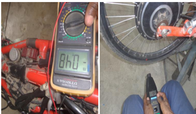
Measuring the current drawn to DC motor by using multimeter
