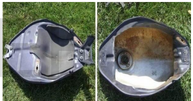
Figure 5. Before and after: fuel tank with bottom removed to make room for components
