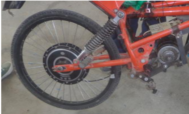
Figure 2. Installed DC motor on the frame
